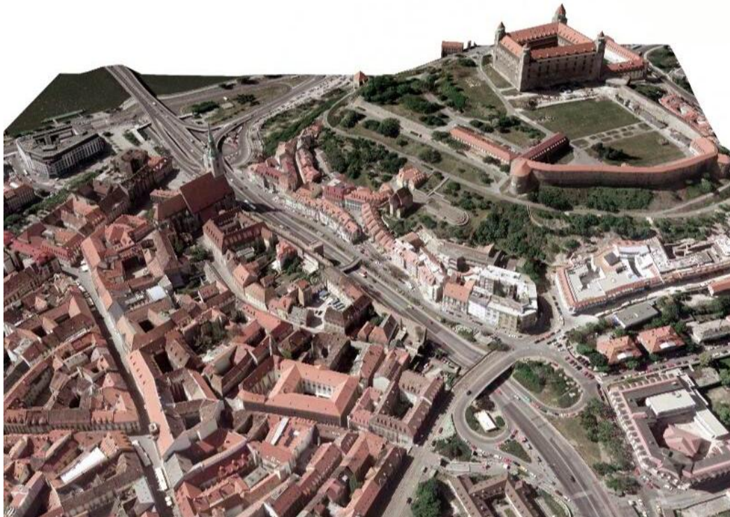
Figure 1: Coarse-detail modeling example – Bratislava Castle and nearby Old Town textured from aerial images.
