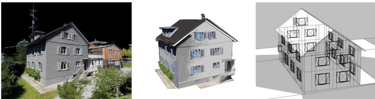
Figure 5: Colorized point cloud from terrestrial laser scanning (left), static 3D building object model based on point clouds (mid), example of a building type generated in the CityEngine system implementing CGA shape grammar rules (right).
