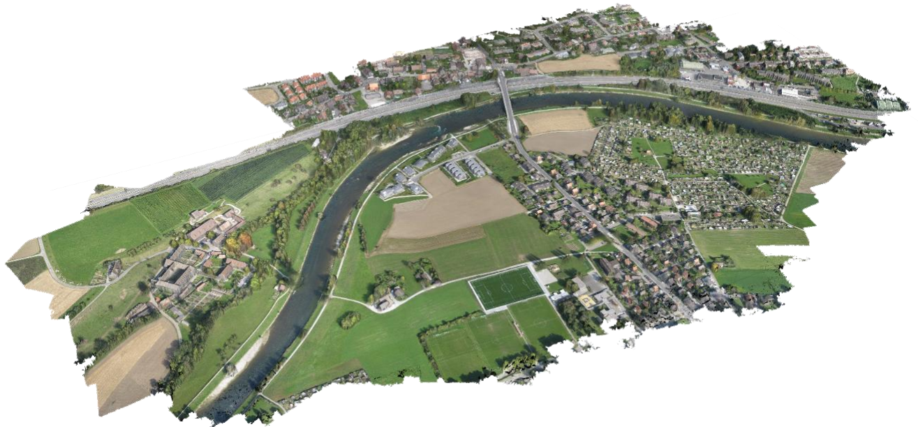
Figure 4: Processed high resolution digital surface model (DSM) with orthophoto texture of an Unmanned Aerial Vehicle (UAV). The data shows a part of the case study area of Schlieren (Canton Zurich, Switzerland) and has an accuracy of 8 centimeters (DSM and orthophoto).
