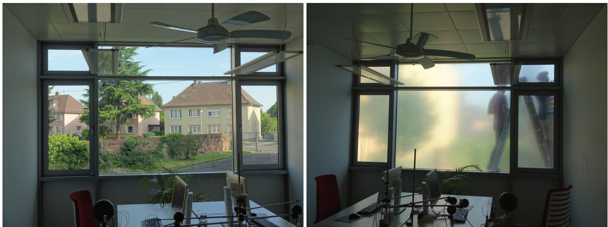
Fig. 2: Experimental set-up of NoiseCon (left: clear view, right: translucent view realized by multiple layers of translucent foil bought at a nearby homecenter for less than 5 €).
