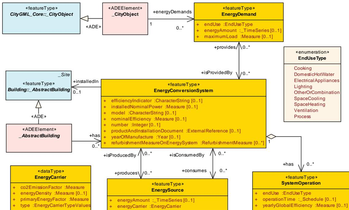
Figure 5: Energy ADE module "Energy system"
