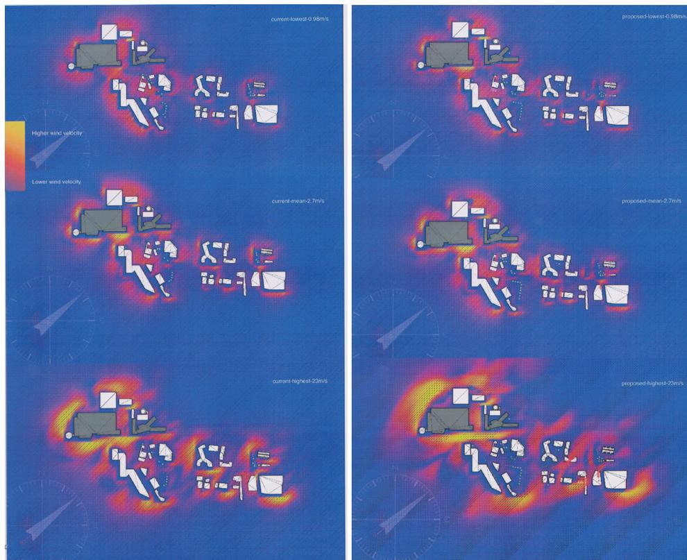
Fig. 6: 2D Vasari Wind Tunnel simulations under current conditions (left) and future conditions (right) for three different wind speeds.
