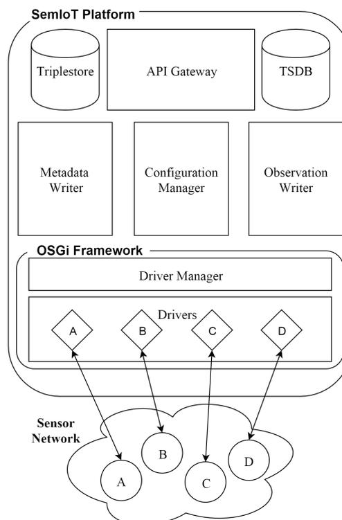
Fig. 3. An architecture of the SemIoT Platform
