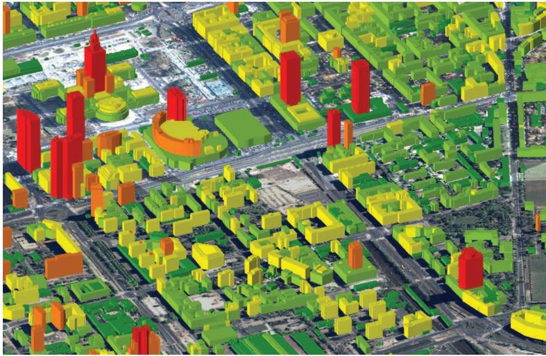
Fig. 3: 3D model of centre of Warsaw, derived from stereopairs of IKONOS satellite, 2005
