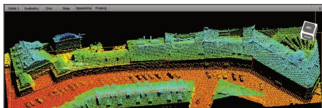
Fig. 12: 3D point cloud from laser aerial scanning (LIDAR data) of ISOK project, Test area 1
