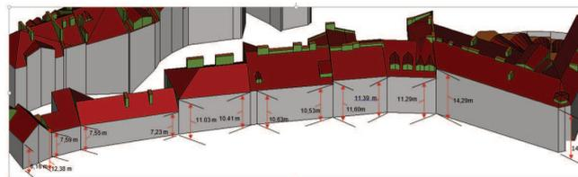
Fig. 11 : 3D model of the Test area 1, derived from stereodigitizing of aerial photos, 2014
