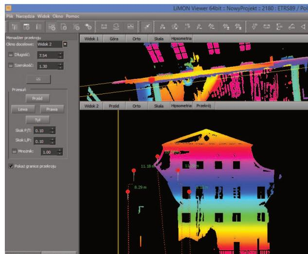
Fig.20: 3D data of terrestrial laser scans are ideal complementary data source for aerial scanning or data derived from stereodigitizing of aerial photos.
