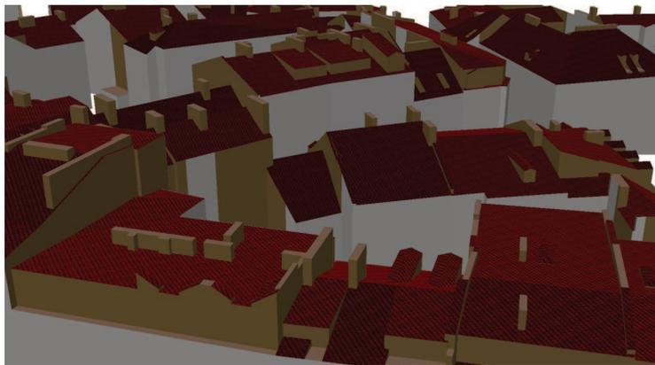
Fig.13: sample model 3D, CityGML LoD 2, with roof details from stereodigitizing
