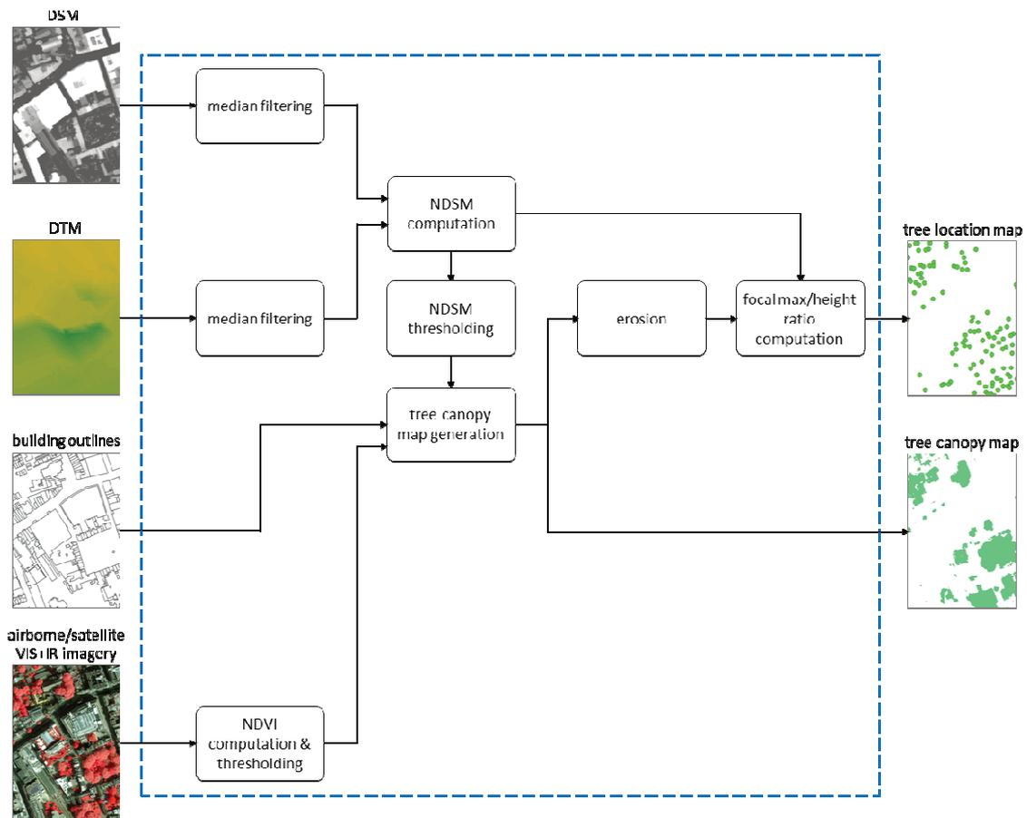
Fig. 5: Block scheme depicting the algorithm developed for mapping tree location and their canopies.
