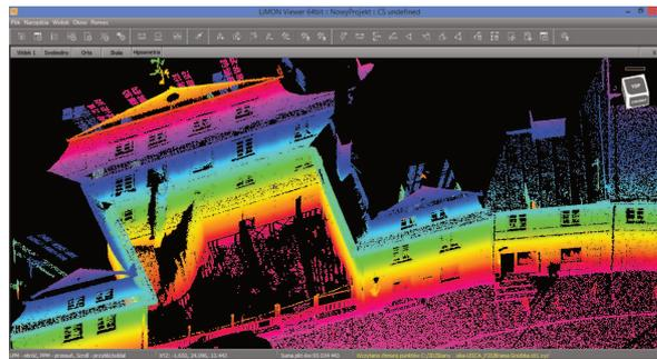
Fig.17: LIDAR from terrestrial scanning are excellent data source for buildings elevation details
