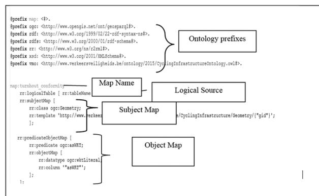
Figure 11: R2RML Mapping: Example of a triplesmap
