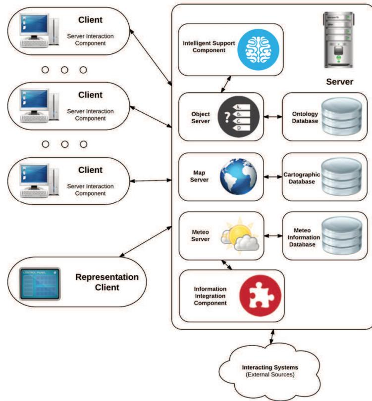
Fig. 1: Situation center's hardware and software complex design.
