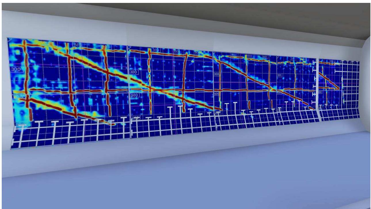
Figure 5: Generic detailed view of a infrared scan inside the bridge of Rosbruck/France (Own source)
