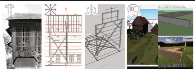
Fig 4: Workflow of creation the shelter, beginning with the site survey, modeling the shelter and visualizing it in Enscape (Esakk and Hermann 2018)
