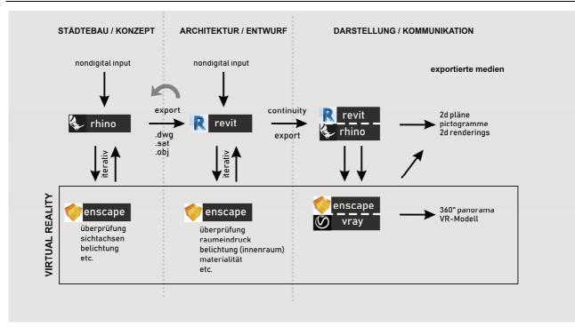
Fig. 1: workflow of using Enscape during the design process and iterative design loops (Maier Chimeno et al. 2018)
