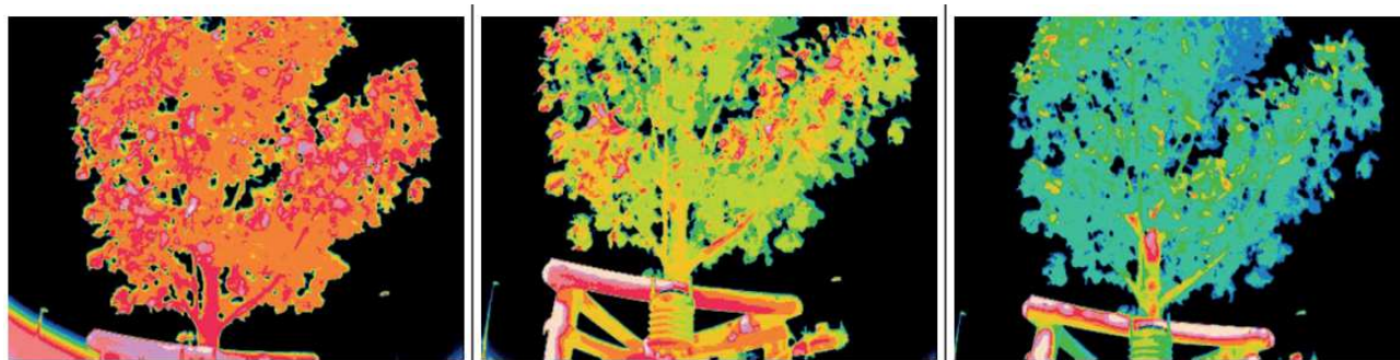
Figure 2: Thermal imaging camera images before rotation (left), during rotation (centre), and after rotation (right). High surface temperatures are represented by red-coloured areas and lower surface temperatures by blue areas [Henninger 2020, p. 76].
